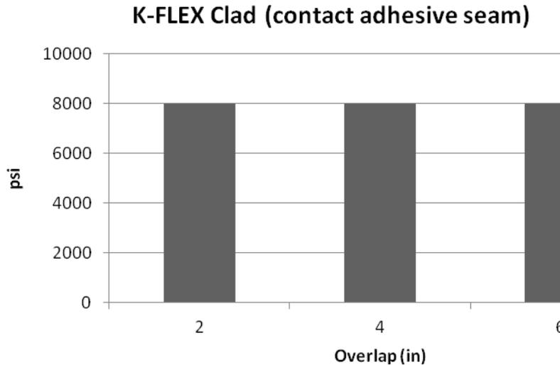
Using a contact adhesive to adhere the seam, the K-FLEX Clad<sup>®</sup> failed before the seam did. All configurations tested the same.
